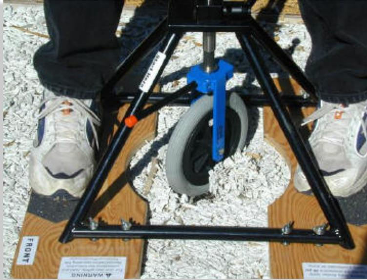
Rotational Penetrometer twisting to measure stability
